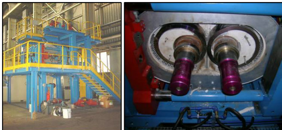
Fig. 5 Roll-diffusion bonding pilot plant (on the left) and detail of the mill stand
